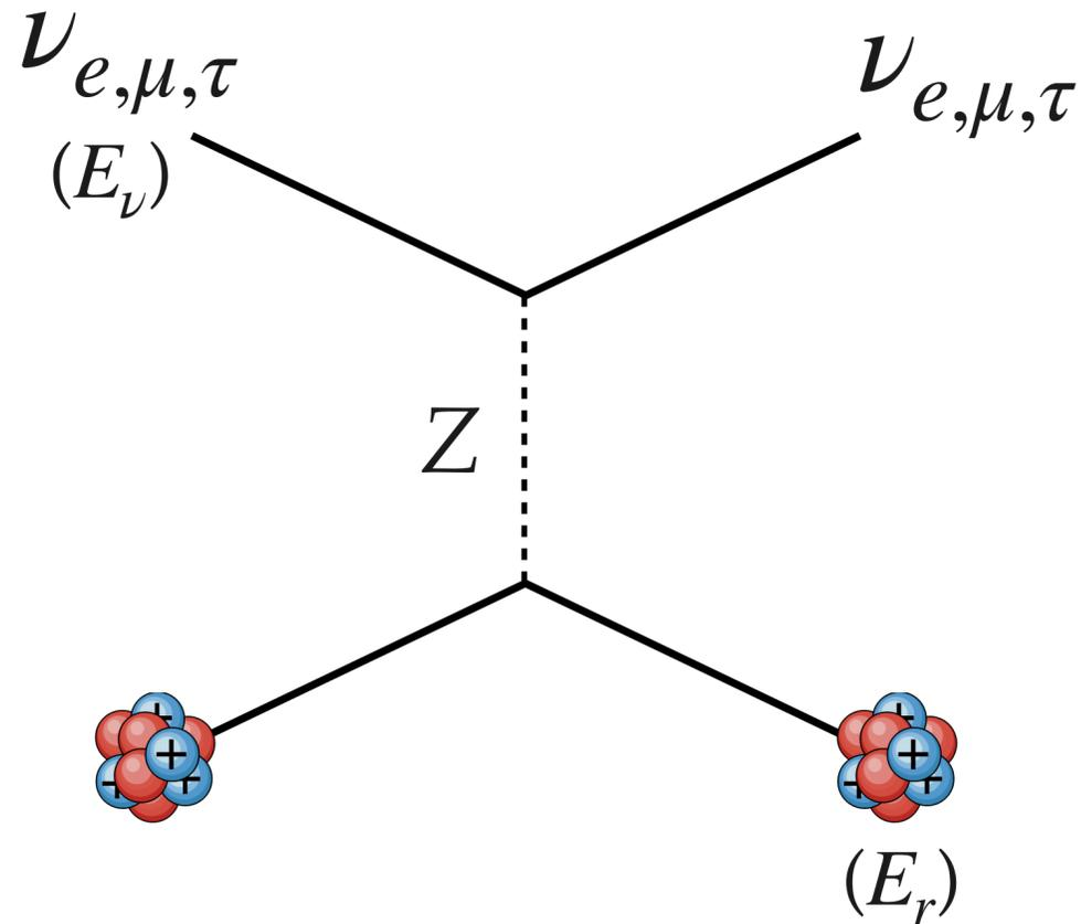
$$\frac{d\sigma}{dE_r} = \frac{G_F^2}{4\pi} \underbrace{Q_W^2}_{\text{Weak hypercharge}} m_N \left( 1 - \frac{m_N E_r}{2E_\nu^2} \right) \underbrace{F^2(E_r)}_{\text{Form factor}}$$
